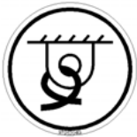
Fig. 7: Label for points used for tying down the machine
