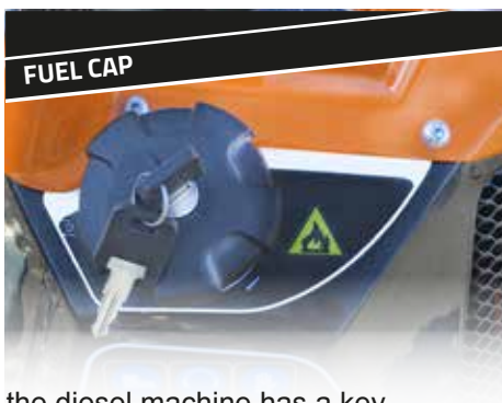
FUEL CAP the diesel machine has a key protected fuel cap
