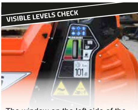
VISIBLE LEVELS CHECK The window on the left side of the unit allow an immediate check of the fuel level
