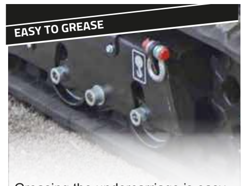
EASY TO GREASE Greasing the undercarriage is easy and fast: nothing has to be taken apart.
