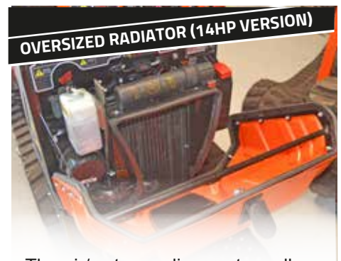
OVERSIZED RADIATOR (14HP VERSION) The air/water cooling system allows the machine to operate in extreme conditions
