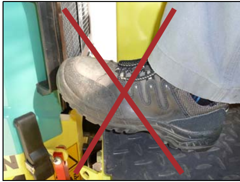
Fig. 7-2 Danger to foot of crushing
