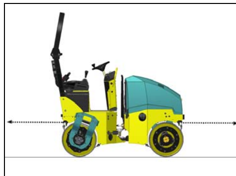
Fig. 9-1 Tow the roller using the towing lugs
