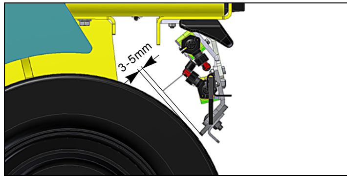
Fig. 9-24 Clearance of scraper to pneumatic wheels
