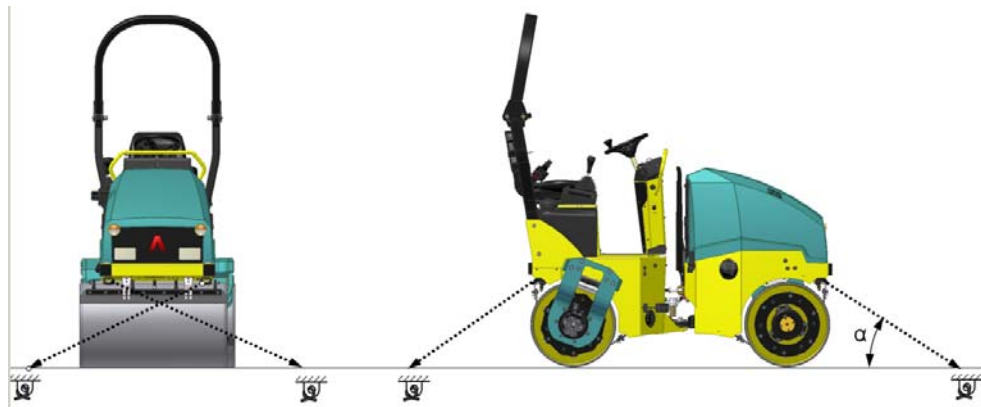
Fig. 12-3 Lashing the roller / side view
