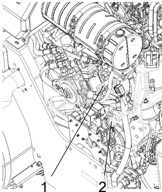
Fig. Engine compartment 1. Forward/Reverse lever 2. Hydraulic reservoir cap
